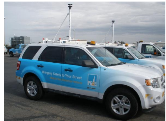
PG&E fleet vehicle with top-mounted leak sensor
