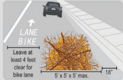
Yard material placement—single-striped bike lane.
