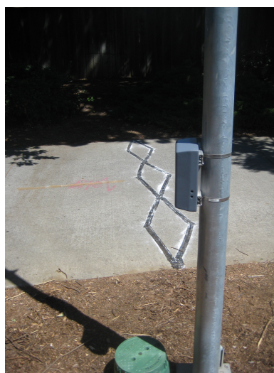
Figure 1: Example of a mobile pyroelectric sensor mounted to a pole.
