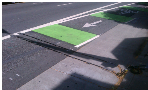
Figure 2: Example pneumatic tubes under use in a bike lane.
