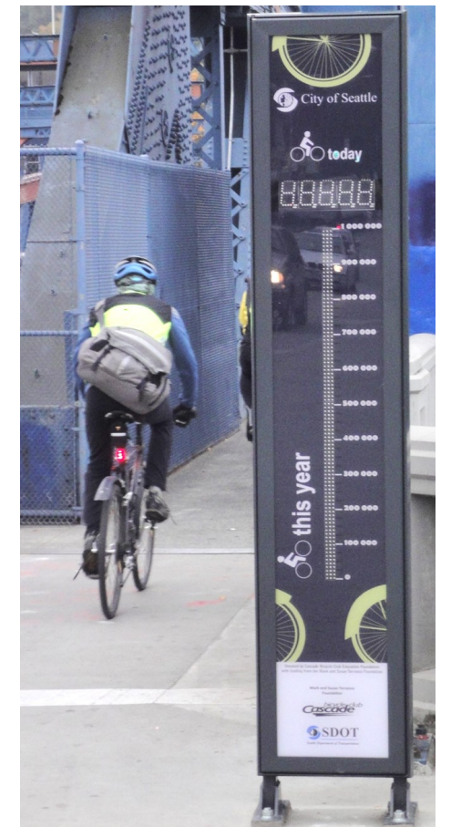
Eco-Totem Counter (Inductive Loop and Display)
