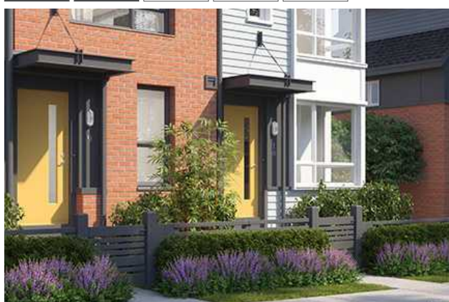
Small Dooryards include low fences to provide a visual transition from the public sidewalk.
