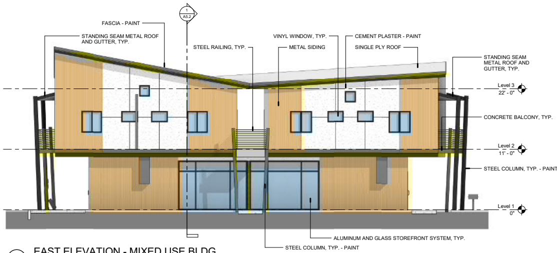
1 EAST ELEVATION - MIXED USE BLDG SCALE: 3/16" = 1'-0"
