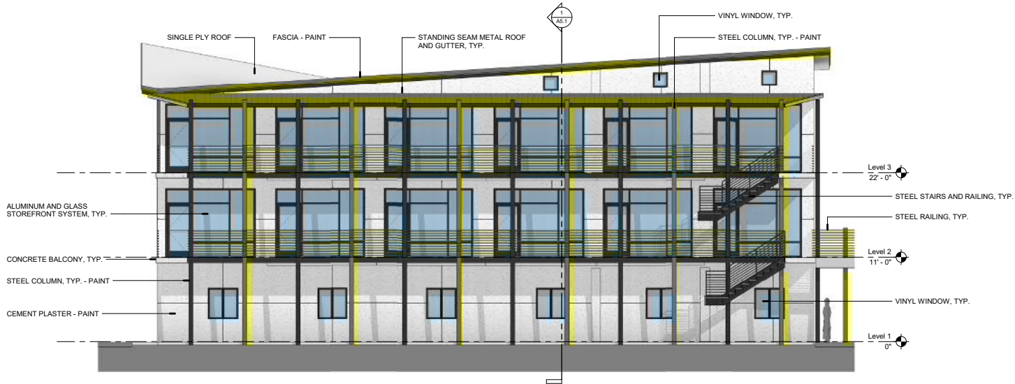
2 NORTH ELEVATION - TYP. RESIDENTIAL BLDG SCALE: 3/16" = 1'-0"
