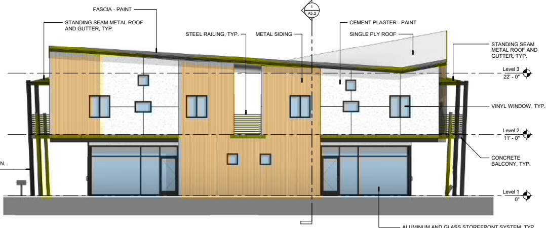
4 WEST ELEVATION - MIXED USE BLDG SCALE: 3/16" = 1'-0"
