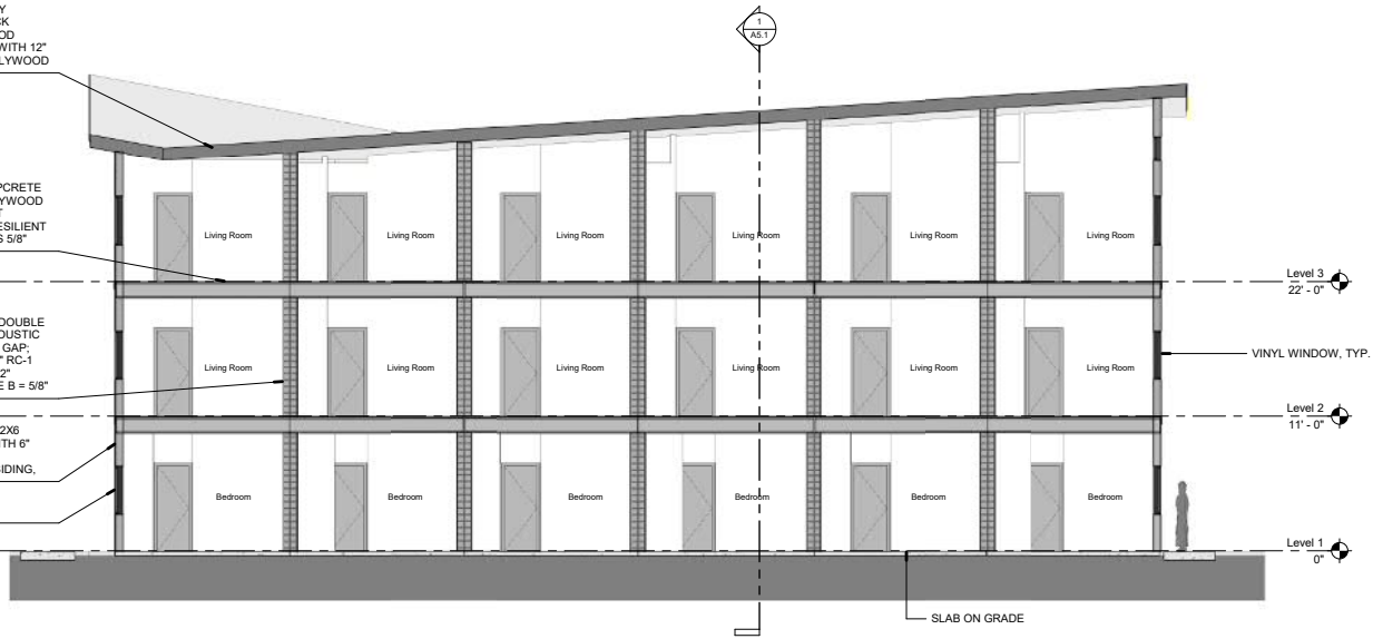
2 LONGITUDINAL SECTION - TYP. RESIDENTIAL BLDG
