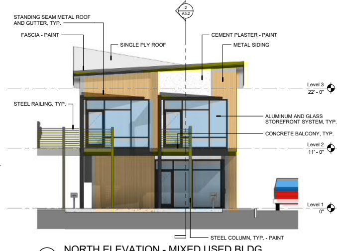
2 NORTH ELEVATION - MIXED USED BLDG SCALE: 3/16" = 1'-0"
