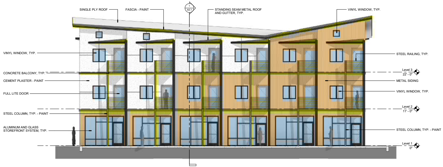
1 SOUTH ELEVATION - TYP. RESIDENTIAL BLDG SCALE: 3/16" = 1'-0"
