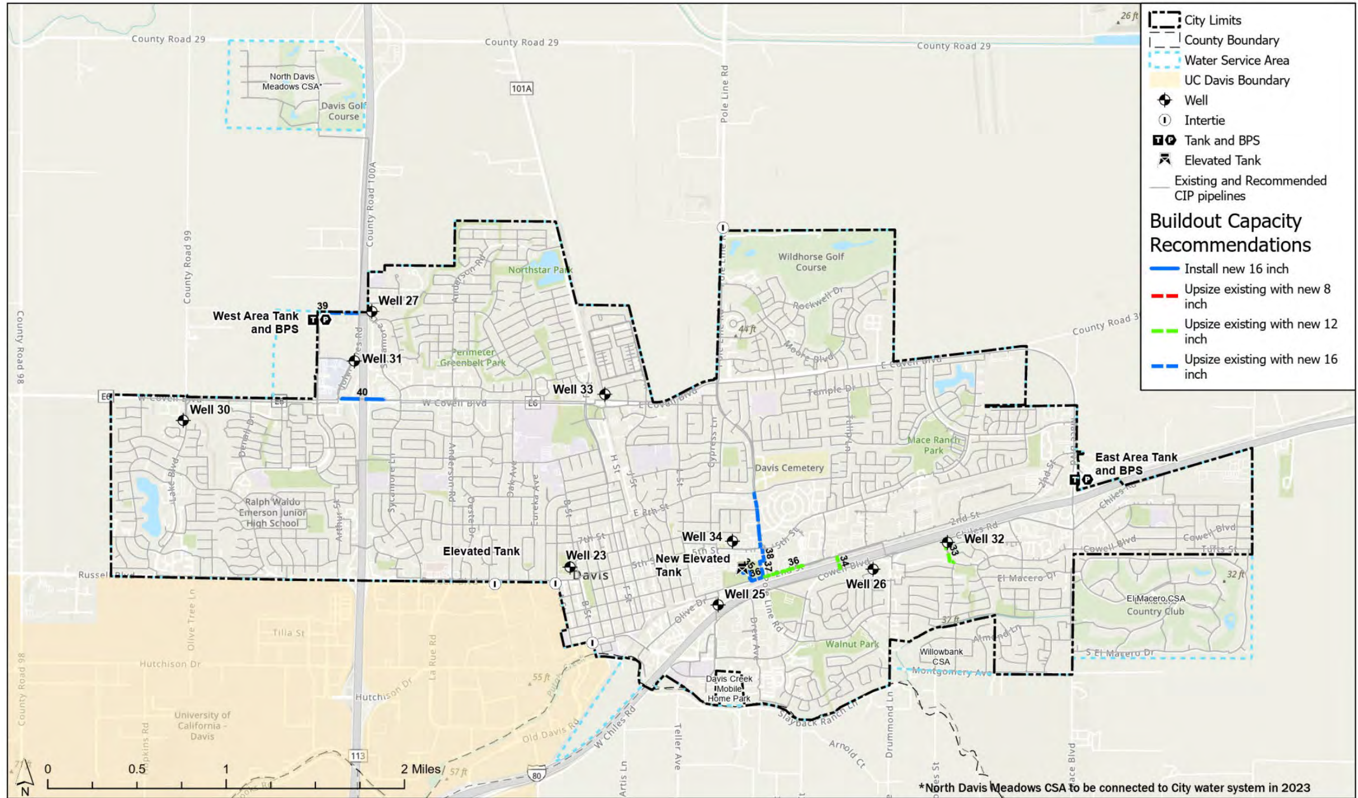
Figure ES-5. Buildout system recommended capacity improvements
