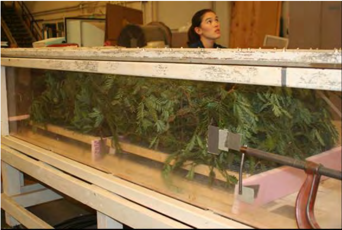
Figure 11 Redwood vegetation in place. Erin monitors wind velocity.
