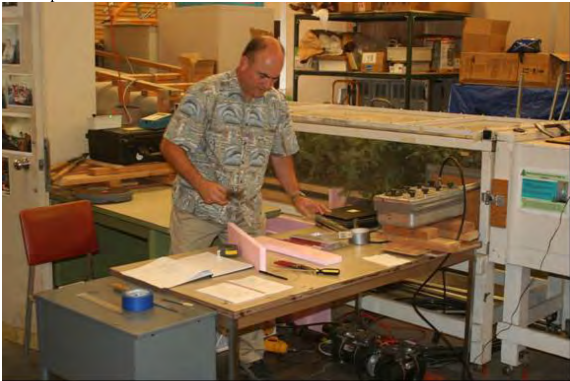
Figure 10 Dave Barnes next to the inlet DRUM and Dustrak, with the vegetation section beside him. The exit DRUM and Dustrak can be seen behind him.
