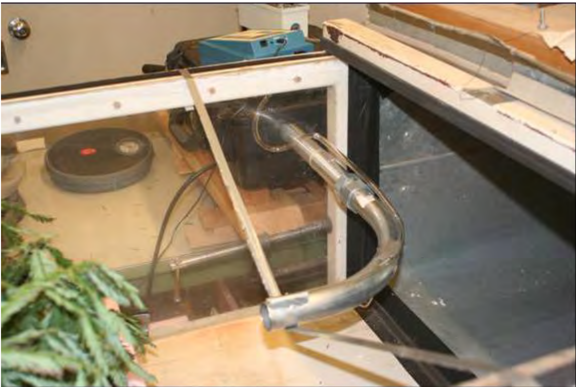
Figure 12 Exit inlets for DRUM and Dustrak.
