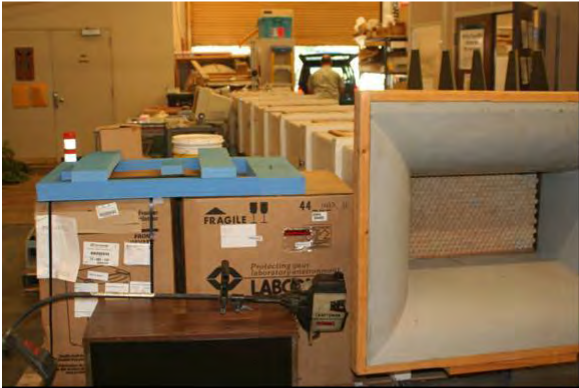
Figure 8 The 60 ft UC Davis low velocity wind tunnel. The collimators on the entrance are shown, then the 20 ft section for flow treatment, and in the distance the end of the tunnel and outside exhaust.
