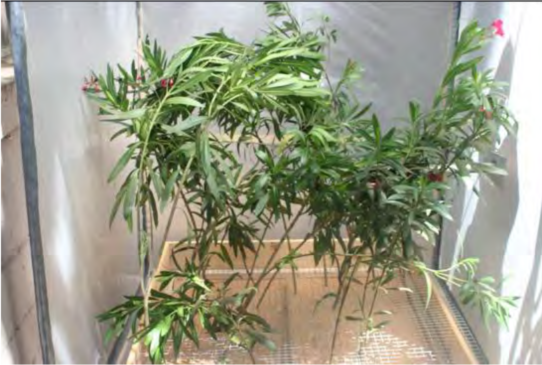
Figure 22 First attempt at vegetation in the static chamber. Even this much oleander absorbed particles so rapidly the chamber could not be filled.
