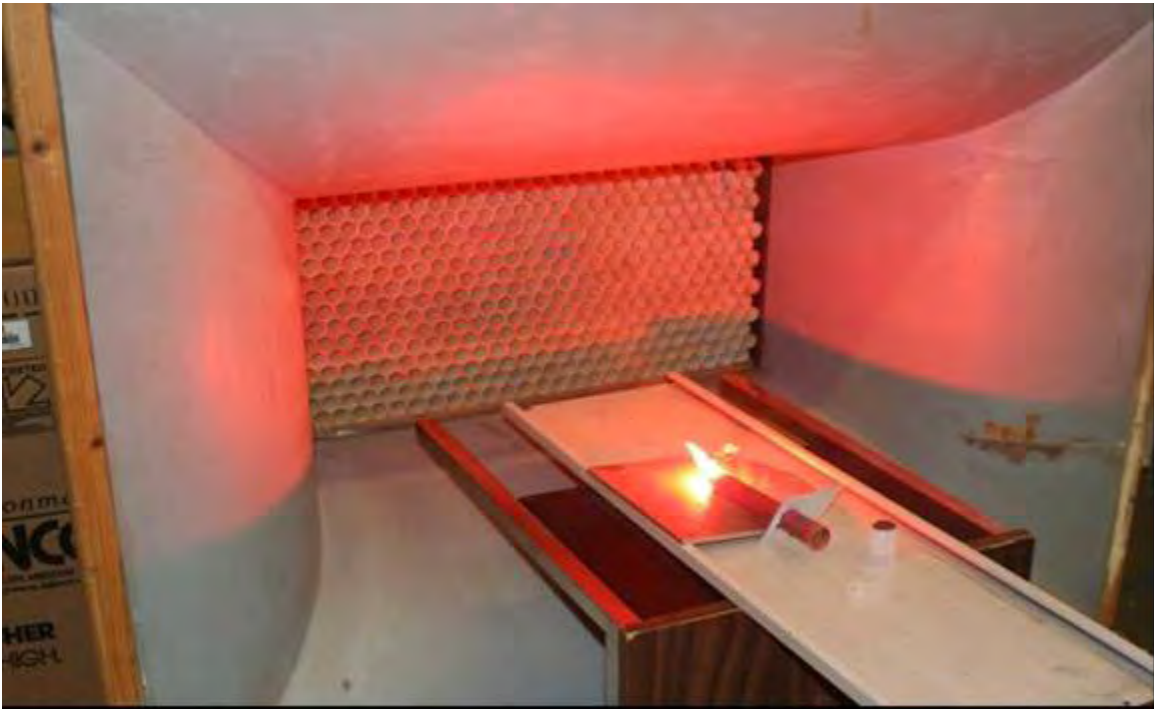
Figure 13 Use of a road flare to generate accumulation mode and very fine aerosol. The flare lasted 15 minutes with the output integrated on the 8 non-rotating stages, inlet and exit. The mean aerosol level before the tests was 13 \mu\text{g}/\text{m}^3 , and in the test 250 \mu\text{g}/\text{m}^3 .
