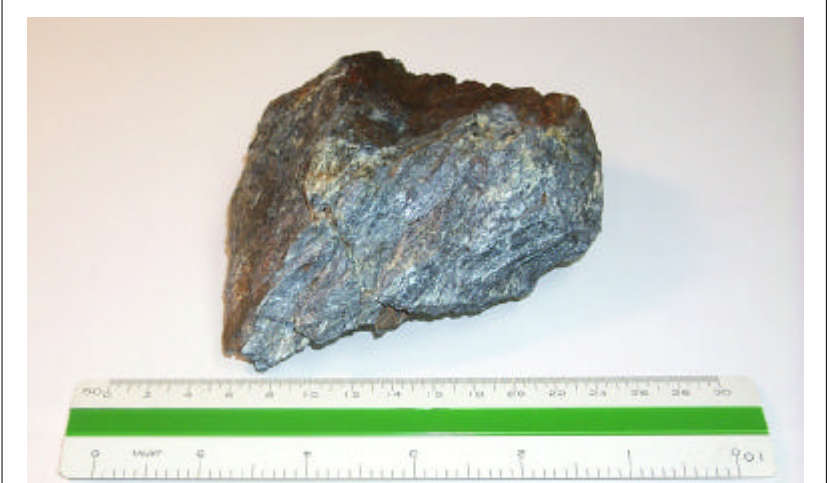
Massive serpentinite, partially to completely serpenitized peridotite (ultramafic rock), with a brown to reddish-brown weathered surface due to oxidation of iron.
