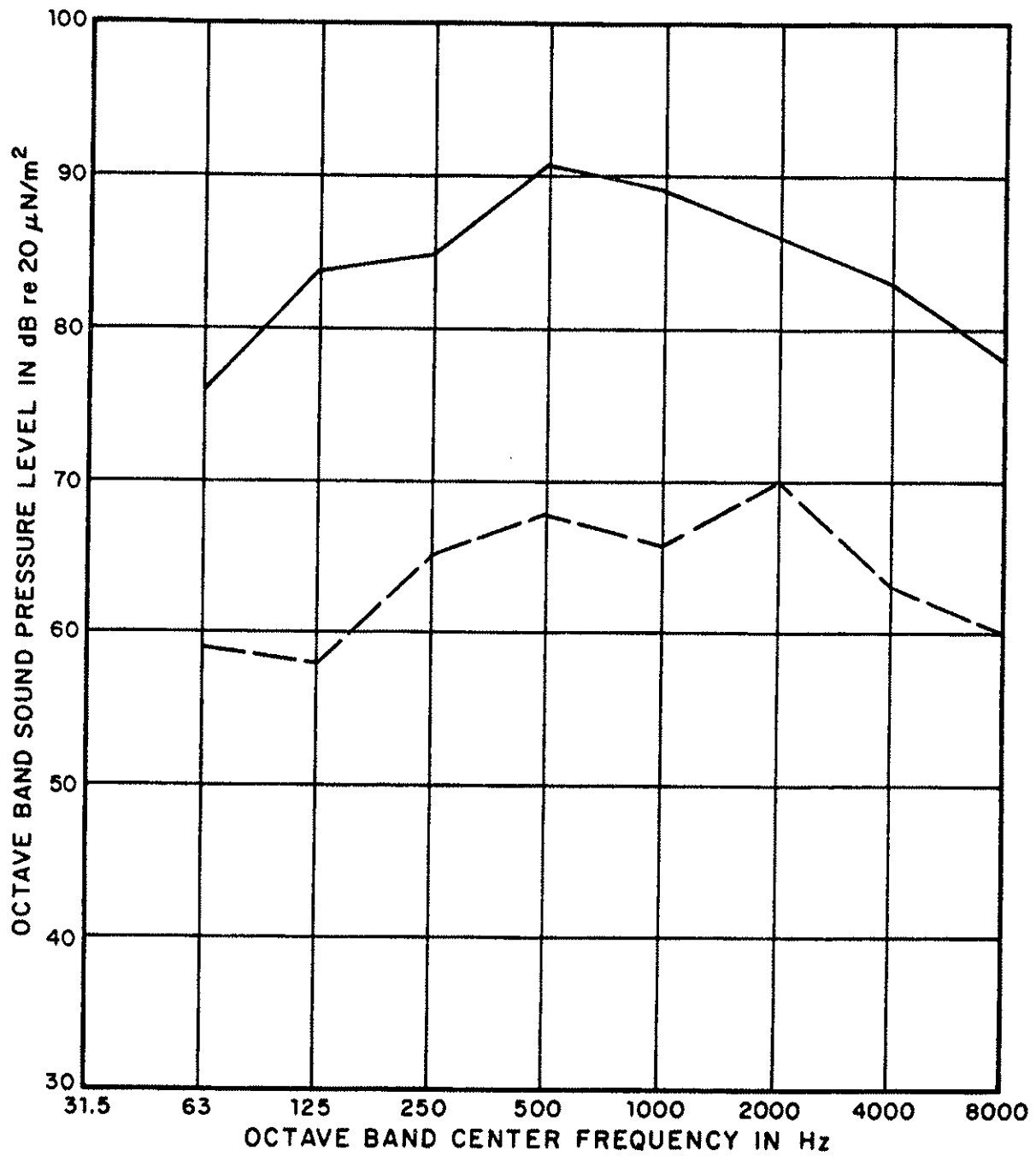
FIG. A.43 RANGE OF SOUND PRESSURE LEVELS FROM PUMPS (MEASURED AT 3 FT)
