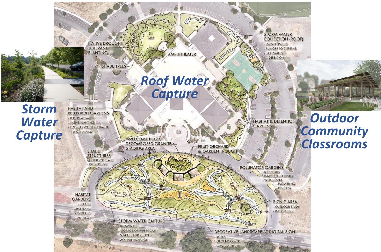
Woodland Community and Senior Center - Water Conservation Improvements
