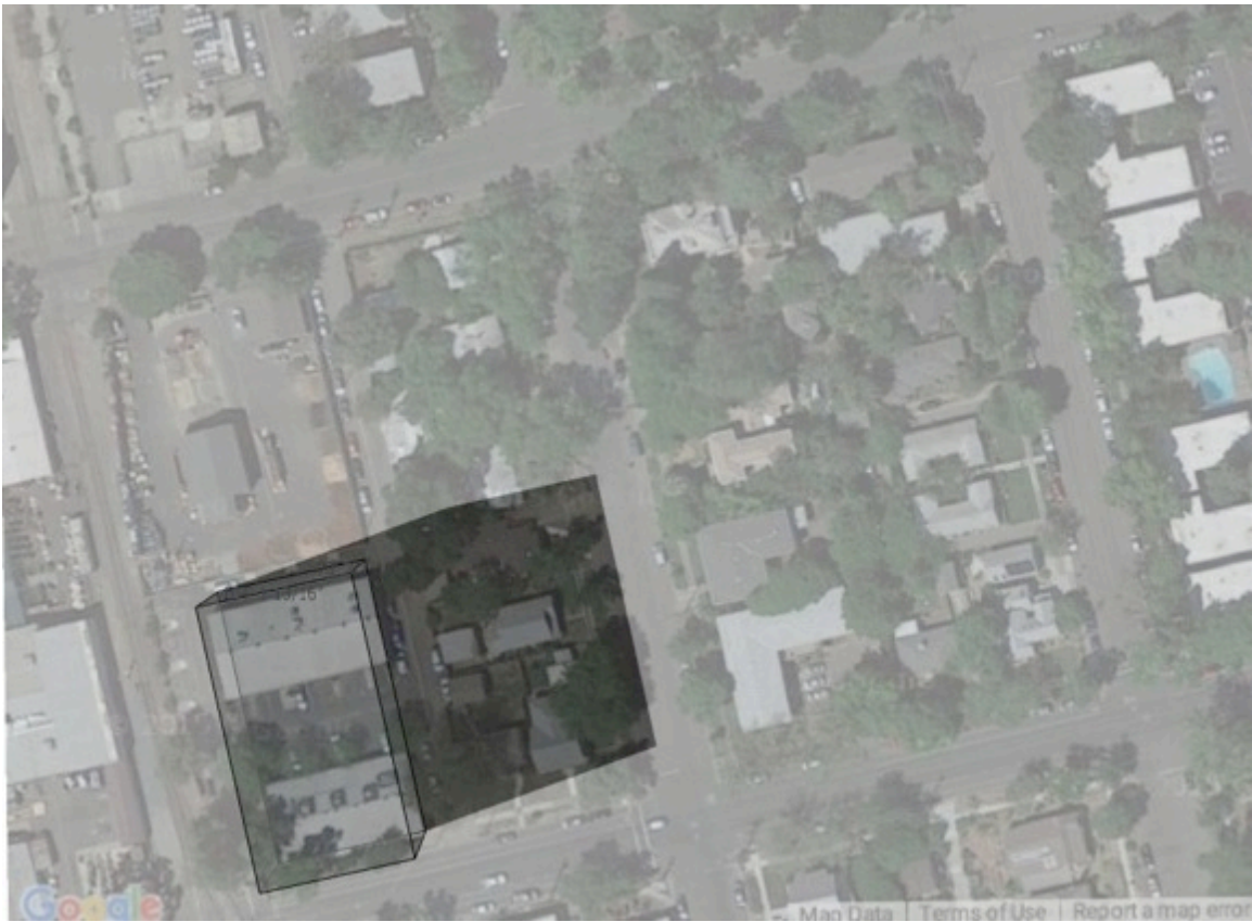
Figure 10: figure generated by the author showing shadow from proposed building at 5 p.m. on September 21 st .
