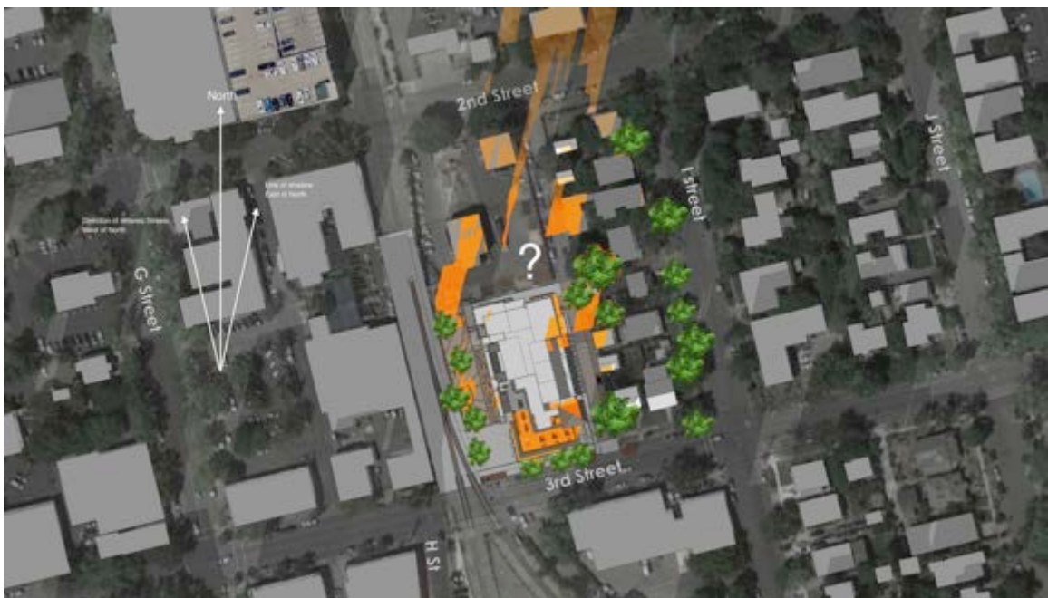
Figure 5: figure from the report showing the shadow from the proposed structure at 4 p.m. on December 21 st . The question mark denotes a strange gap in the computed shadow.
