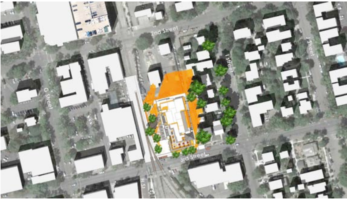
Figure 9: figure from the report showing the shadow from the proposed structure at 3 p.m. on September 21 st .
