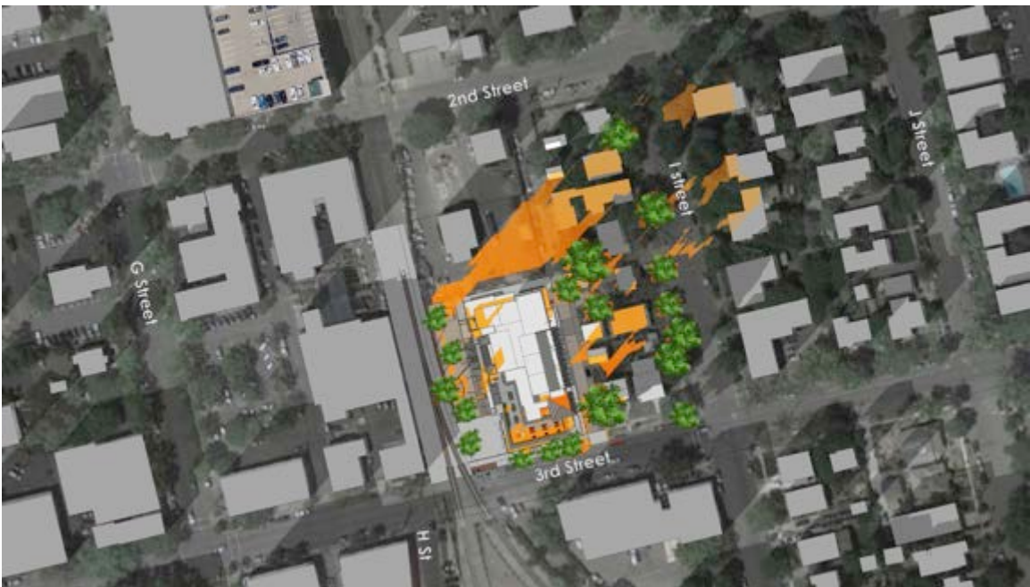
Figure 11: figure from the report showing the shadow from the proposed structure at 5 p.m. on September 21 st .5 p.m.
