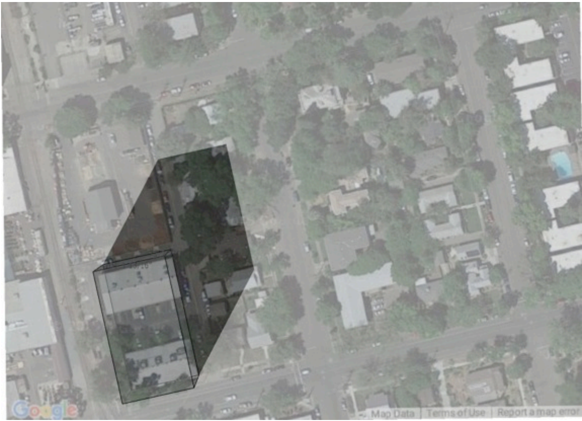
Figure 6: figure generated by the author showing shadow from proposed building at 2 p.m. on December 21 st .
