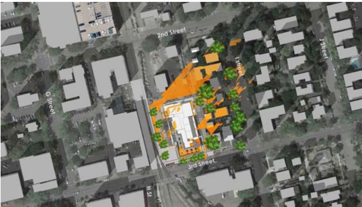
Figure 15: figure from the report showing the shadow from the proposed structure at 5 p.m. on June 21 st .
