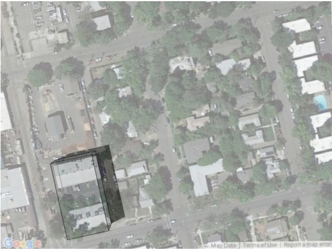
Figure 12: figure generated by the author showing shadow from proposed building at 3 p.m. on June 21 st .
