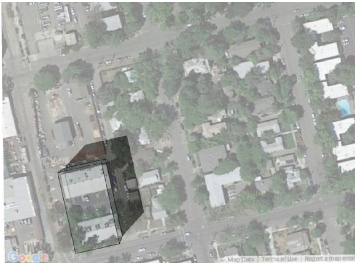
Figure 8: figure generated by the author showing shadow from proposed building at 3 p.m. on September 21 st .
