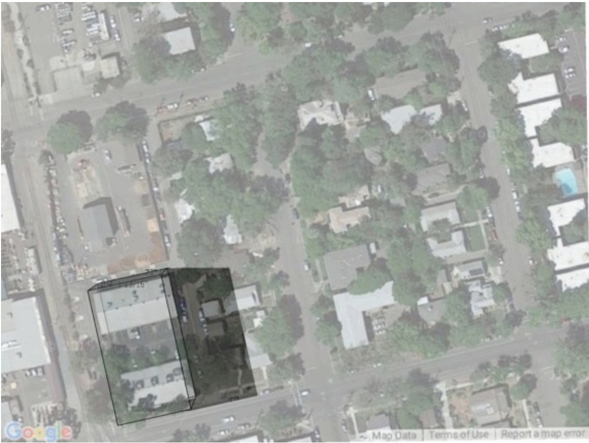
Figure 14: figure generated by the author showing shadow from proposed building at 5 p.m. on June 21 st .
